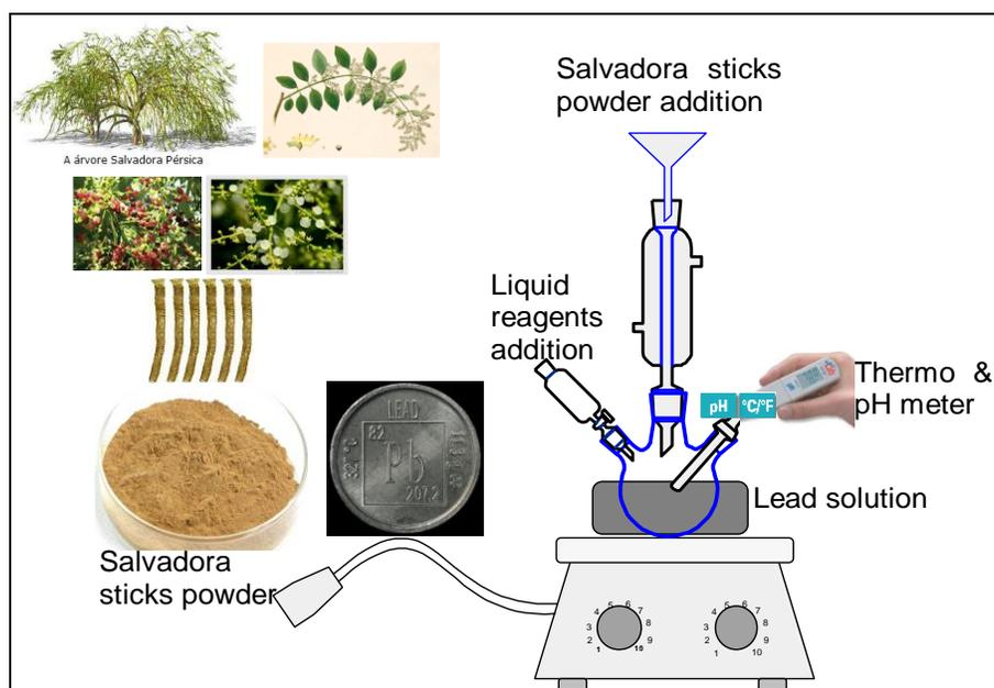
**Figure 1:** Graphical concept for mitigation of lead ions from aqueous media using *Salvadora persica* as biosorbent material.
