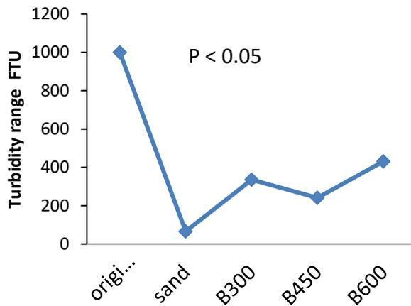
**Figure 4.** Changes in turbidity values before and after the treatment with the adsorbents.
