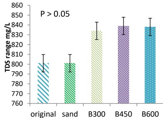
**Figure 3:** Mean value of TDS after the treatment with sand and wastewater compared using one way ANOVA (n=3).
