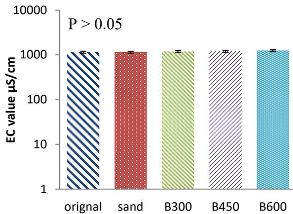
**Figure 2:** Comparison in means of original sample, sand treated wastewater samples and biochar treated wastewater samples, showing a trend in change of EC before and after the treatment.
