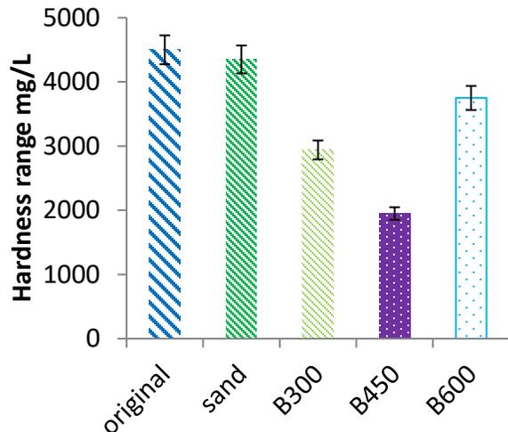
**Figure 6.** Trend showing reduction in total hardness before and after the adsorption process.
