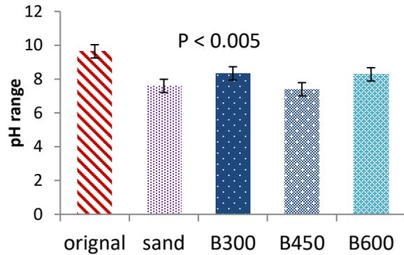
**Figure 1:** Trend showing the changes in pH before and after the treatment and difference in pH changes between sand and biochar samples as well as different biochar samples.
