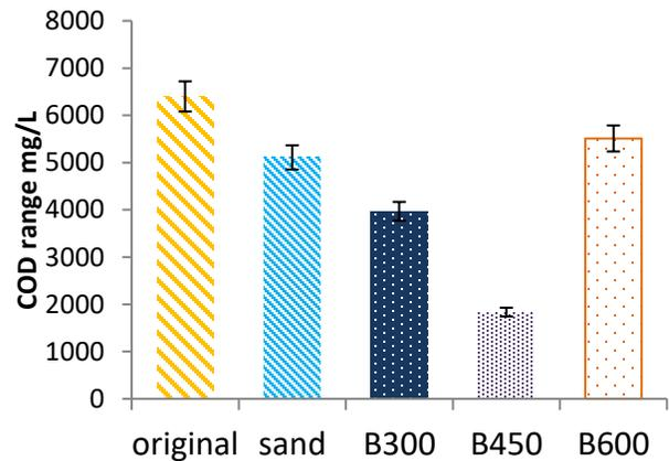
**Figure 5.** Trend showing difference in the COD value of the treated samples compared to the original sample.
